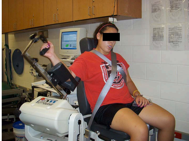
Figure 2. Proper set up of Biodex System 3 dynamometer for the shoulder exercises.
